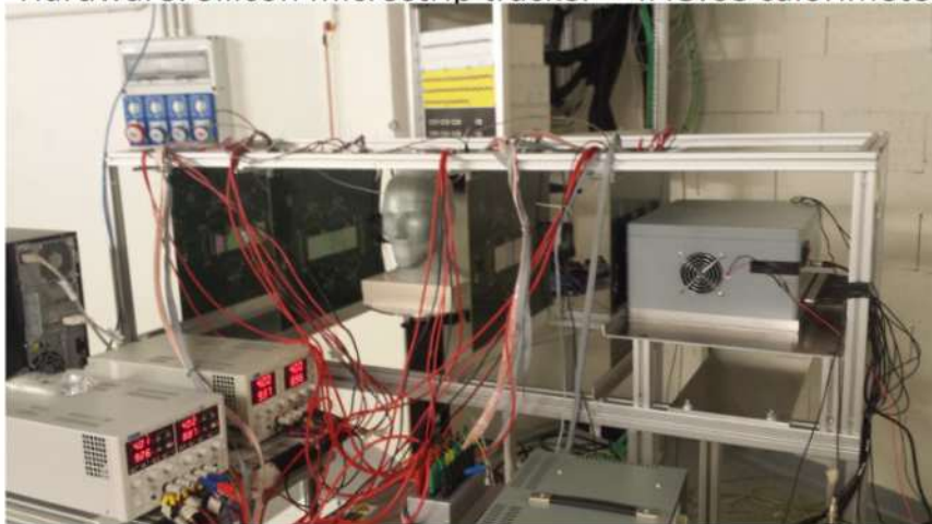
INFN pCT system under test with an anthropomorphic head phantom at Trento proton therapy center's experimental beam line
