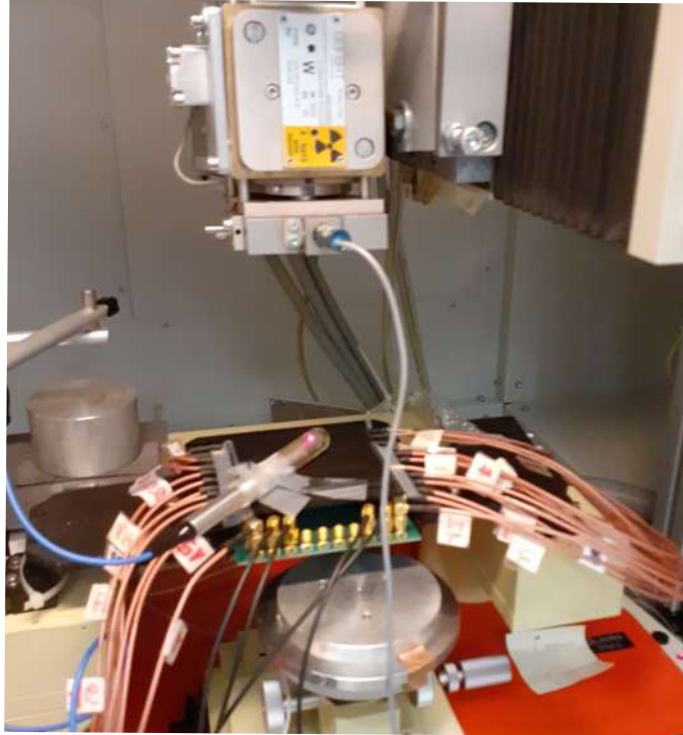
Calibrated diode/PTW farmer chamber Comparison in the Padova laboratory
