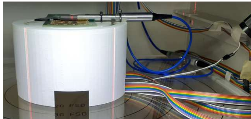
Farmer chamber and SiPM support (FBK)
