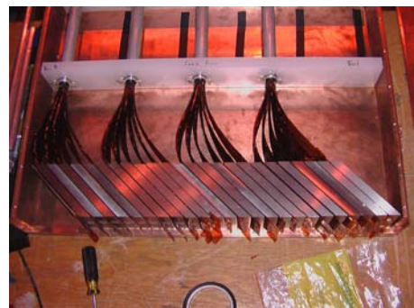
Figure 6.5: Photograph of the ZDC HAD section.
