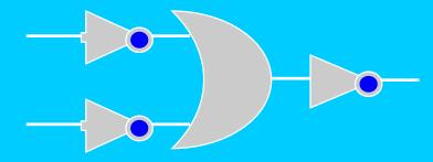
One can test explicitly that this device has an identical truth table as the AND gate.
