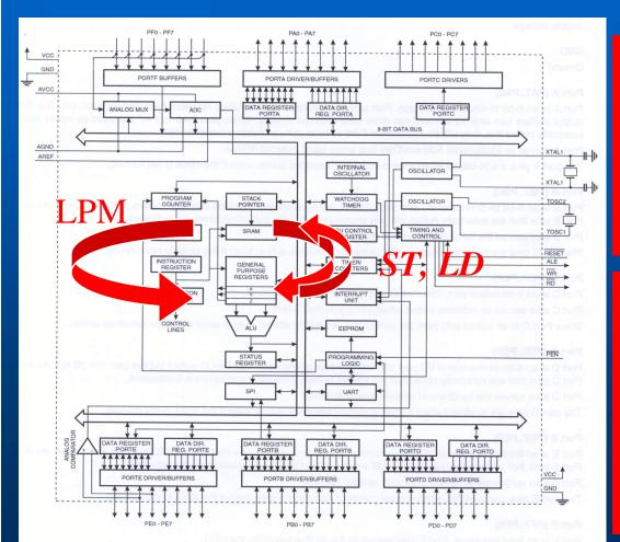
This way data can be moved from the data SRAM to the register file and the reverse using LD and ST commands
