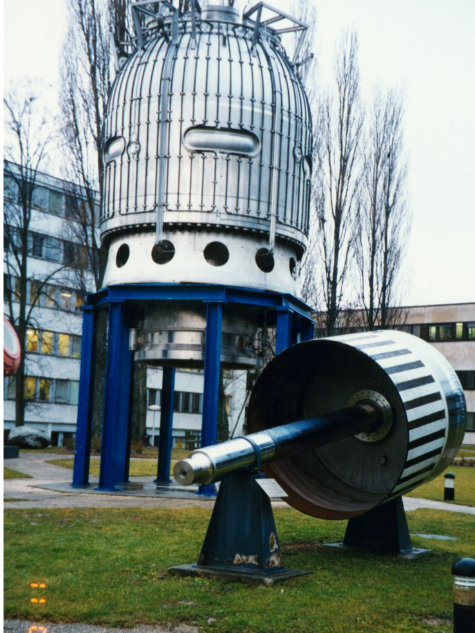
Figure 16: The Big European Bubble Chamber and its piston at CERN after being decommissioned.
