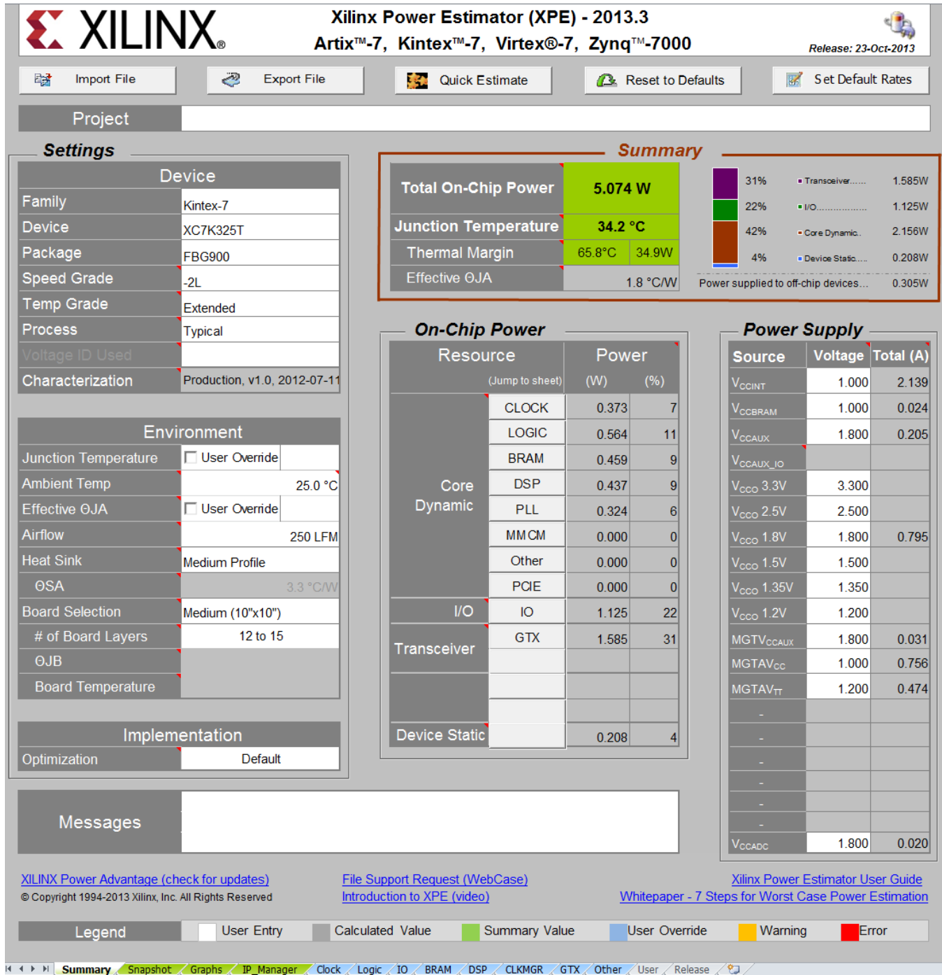
Figure 21: Summary Sheet (Kintex-7) - Adjust Settings and Display Power Results
