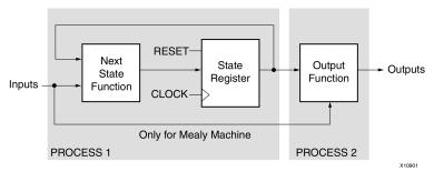
A Finite State Machine (FSM) With One Process can be described with three processes using the FSM decomposition shown in the following diagram.
