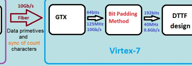
Two options are used to design the new transceivers, synchronous and asynchronous. At the asynchronous mode a Bit Padding Method is used.
